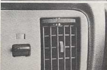
Left: the air vents — one at each end of the fascia, two in the middle — are very effective but they whoosh and hiss when open. Right: simple but stiff heater controls, clear minor switchgear
