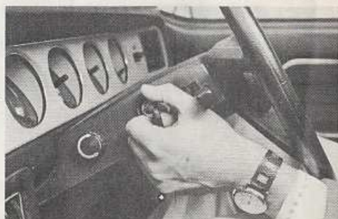
Left: unusual "dagger" key (handy as a defensive weapon, painful if you sit on it) works the locks of all four doors with one twist. Right: it is hard to turn the ignition key without nudging the adjacent wiper stalk. The aim of the headlights can be adjusted by knurled knob
